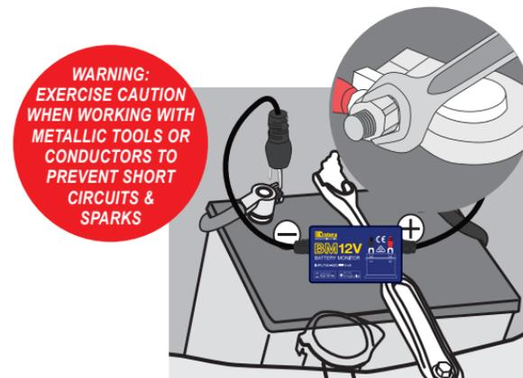
1. Attach Red connector to the Positive (+) battery terminal and the Black connector to the Negative (-) battery terminal.
