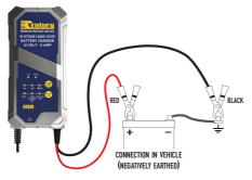
If Negatively Earthed (Most Common) — FIRST Connect the Red (+) Crocodile clip or ring terminal lead to the (+) battery terminal and then connect the Black (-) Crocodile clip or ring terminal lead to the vehicle's chassis. DO NOT connect the Black (-) lead to the carburettor or fuel lines.
