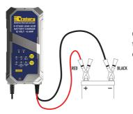
Connect the Red (+) Crocodile clip or ring terminal to the (+) battery terminal. Connect the Black (-) Crocodile clip or ring terminal to the (-) battery terminal.
