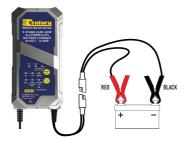
Connect the Red (+) crocodile clip or ring terminal to the (+) battery terminal. Connect the Black (-) crocodile clip or ring terminal to the (-) battery terminal.
