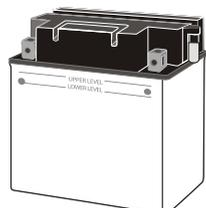
6. Loosely replace refilling plugs to avoid electrolyte spitting while charging.
