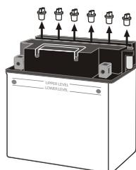
3. Remove electrolyte bottle, cut the tip of the cap in half, and connect one end of the orange tube to the cap and the other end of the orange tube to one of the battery cell holes as shown.
