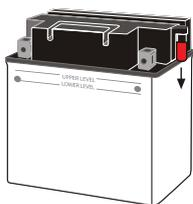
2. Remove filling plugs located on battery top. And connect transparent exhaust pipe to the battery exhaust nozzle.
