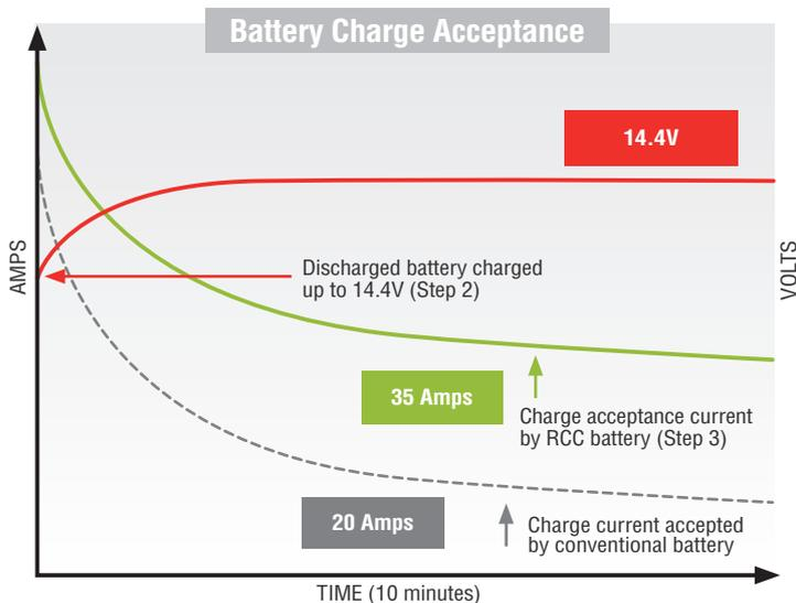
The higher the charge rate accepted by the battery, the better the battery will work in conjunction with a vehicle's alternator and battery management system to reduce fuel consumption and vehicle emissions. Batteries optimised for vehicles fitted with RCC systems can achieve up to 8% higher charge acceptance than conventional batteries.
