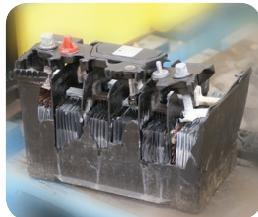
During operation and charging, lead acid batteries produce hydrogen and oxygen which occupies the headspace in a battery above the electrolyte. If such gasses are not vented correctly or are exposed to a source of ignition, battery explosion can occur. In order for a battery to explode two elements must be present – explosive gasses, namely hydrogen and oxygen, plus a source of ignition, external or originating from within the battery.
