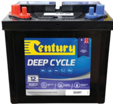
Century Deep Cycle Flooded batteries are constructed using thicker plates, specialist antimonial lead alloys and denser active material, to withstand repeated recharge and discharge cycles. The maintainable design enables easy access and topping up of electrolyte levels for maximum control over battery life. Premium grade raw materials and electrolyte ensure reliable deep cycle performance in recreational and commercial applications.
